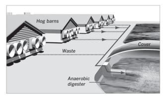
**Waste is flushed** from hog barns into a covered pond called an anaerobic digester, where bacteria "digest" the waste and produce methane gas.
