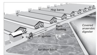
**Liquid waste then flows into an aeration basin**, which treats the water for pollutants such as ammonia. The water can then be reused for irrigation and barn-flushing.
